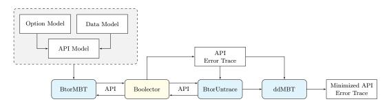
Figure 1: General workflow of model-based API testing for Boolector.
