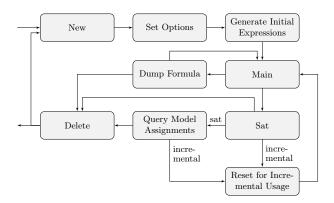
Figure 2: The API model of Boolector as implemented in BtorMBT.
